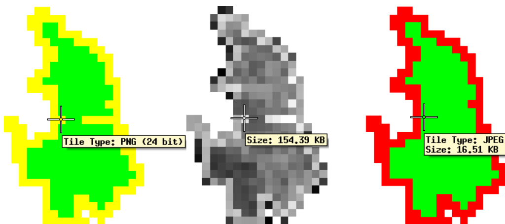
Zoom level 13 tile map (left) and stored tile size map (right) for the national parks tileset. This tileset was created using the option for 24-bit PNG tiles (yellow) instead of 8-bit PNG for edge tiles. While most fully-opaque interior tiles are in JPEG format (green), a few interior tiles are in 24-bit PNG format; DataTips for one such interior tile are shown. These opaque PNG tiles have much larger stored sizes than equivalent JPEG tiles, and would thus require longer download times, slowing the display of the tileset in a geobrowser.
