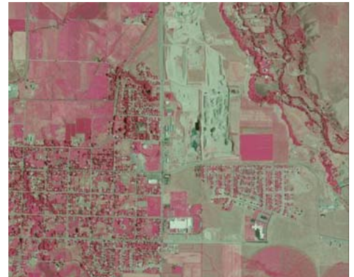
Detail of 1-meter resolution color-infrared orthoimage hierarchical tileset with zoom levels 13 through 17 covering the same county.
